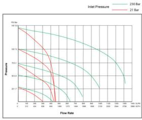
"FLOW TAKEN UNDER STANDARD WORKING TEMPERATURE OF 25"C +-1.1"C USING OIL FREE BREATHABLE COMPRESSED AIR, WITH DIGITAL FLOW DEVICE (SERVAL NO.99753) GALBERATED TO FULL SCALE PRESSURE 140P3IA WITH AN ACCURACY OF +-1.0.5% OF FULL SCALE PRESSURE.
