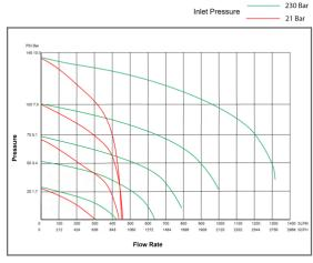
\*FLOW TAKEN UNDER STANDARD WORKING TEMPERATURE OF 25°C +/- 1.5°C USING OIL FREE BREATHABLE COMPRESSED AIR, WITH DIGITAL FLOW DEVICE (SERIAL NO.80763) CALIBRATED TO FULL SCALE PRESSURE 160PSIA WITH AN ACCURACY OF +/- 0.5%, OF FULL SCALE PRESSURE.
