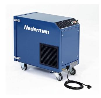
The FE 24/7 1.5 is a mobile high vacuum unit designed to extract welding fumes in a continuous basis. Connected to a welding torch with integrated extraction or to an extraction nozzle, the FE 24/7 1.5 unit extracts the fumes directly at source. Automatic filter cleaning, side channel fans with high capacity and all special values that a Nederman product offers.
