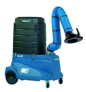
FilterCart Original mobile filter unit for light welding and extraction applications. FilterCart Original includes Extraction Arm Original with an integrated spotlight, which optimizes the user-friendly design. If a larger working range is needed, the 3 m (10 ft.) long arm is recommended.
